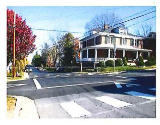
Photo – This is an example of a raised intersection with raised pavement surface and pavement markings that force drivers to slow as they approach the intersection and provide more driver awareness to their speed and need to comply with stop signs.
