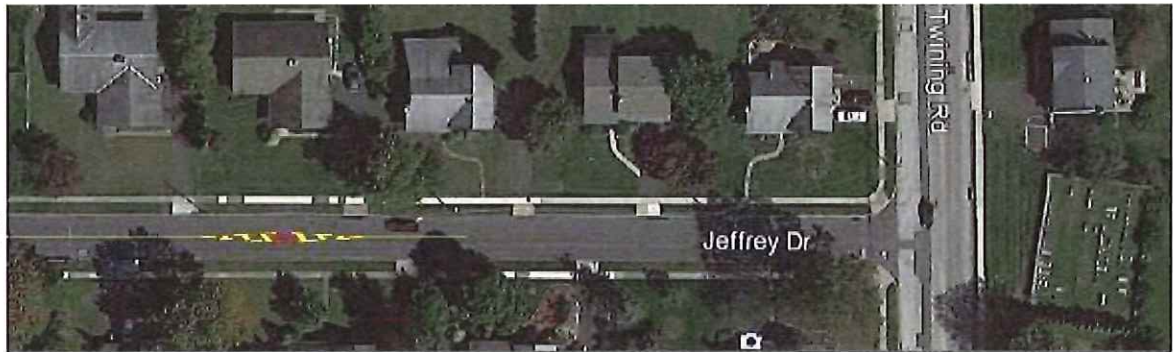
Figure 1 – Yellow pavement markings are proposed to introduce a double yellow centerline and install thick yellow gore markings at two locations to narrow the travel lanes. The areas shown in red are the outlines where ground-mounted delineators will be installed to define the narrowed lanes.
