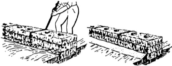
A Rock Construction Entrance is installed along the roadway for the purpose of cleaning mud from the tires of construction vehicles before they leave the worksite. (Figure 3)
