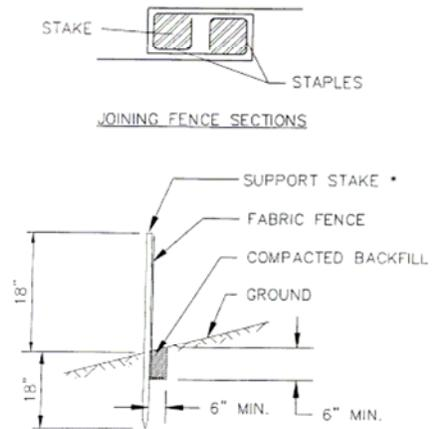
\*Stakes spaced @ 8' maximum. Use 2" x 2" wood or equivalent steel stakes.
