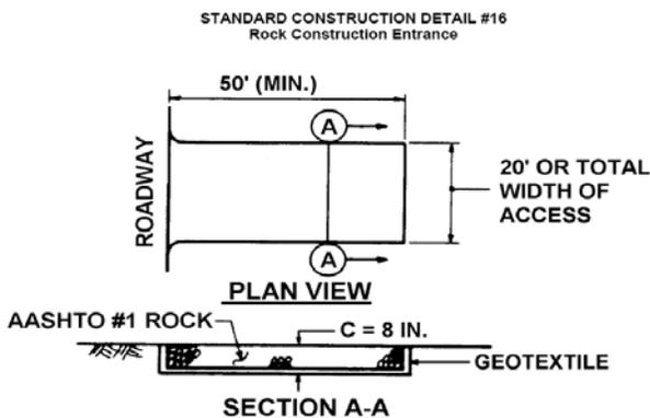
**MAINTENANCE:** Rock Construction Entrance thickness shall be constantly maintained to the specified dimensions by adding rock. A stockpile shall be maintained on site for this purpose. At the end of each construction day, all sediment deposited on paved roadways shall be removed and returned to the construction site.
