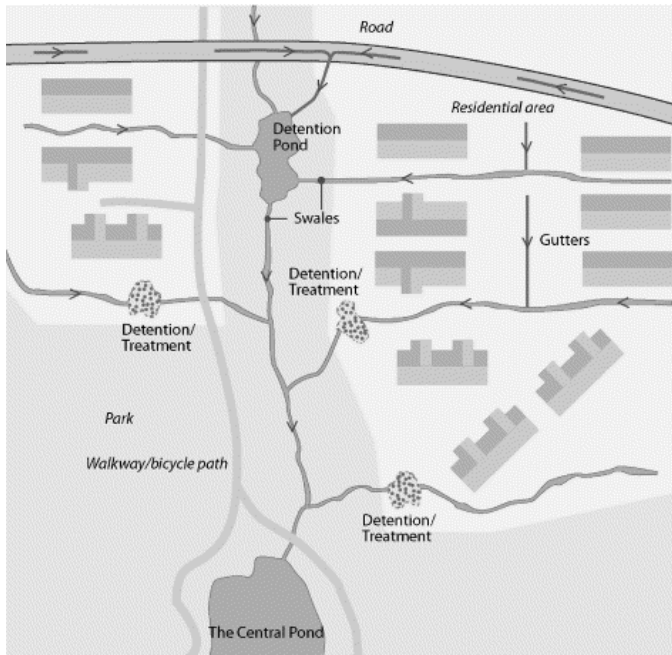
Stormwater Layout for Fornebu showing large central pond, detention treatment ponds near road and roof areas, open channels and central pond (Åstebøl, et.al., 2004)
